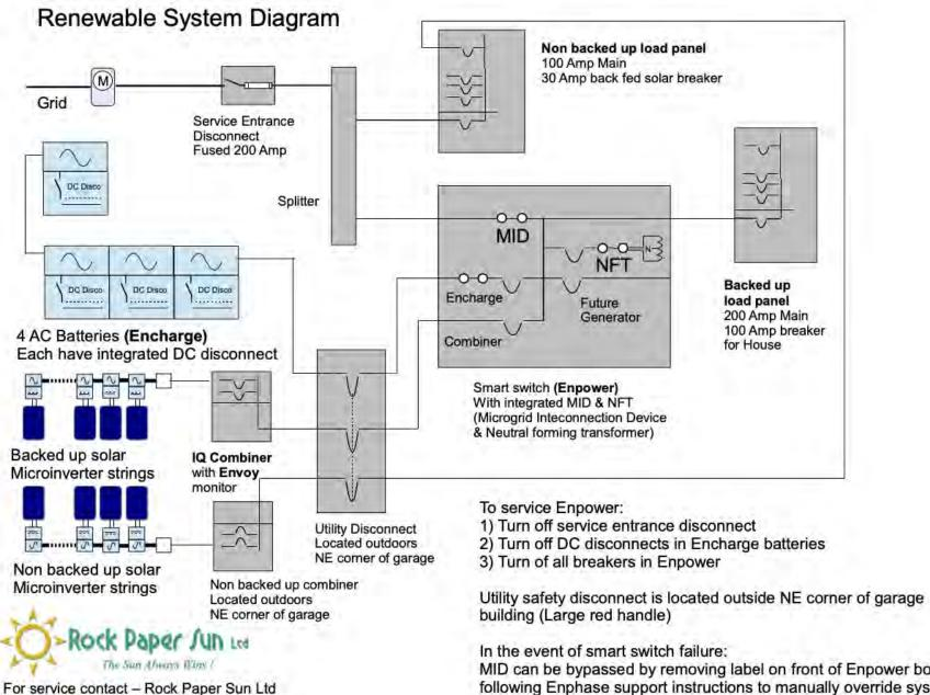
MID can be bypassed by removing label on front of Enpower box and following Enphase support instructions to manually override system
